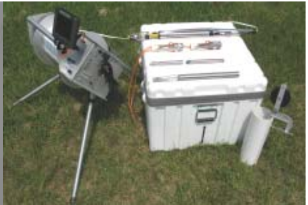
The deluxe winch, the micro camera, the nano camera with motorized side looking mirror, the standard camera, the Jr camera, the motorized pan and tilt with a standard camera. They are resting on top of the deluxe carrying case which is 26 x 26 x 22 inches and foam lined. The encoder wheel and cable protector is to the side of the case.
