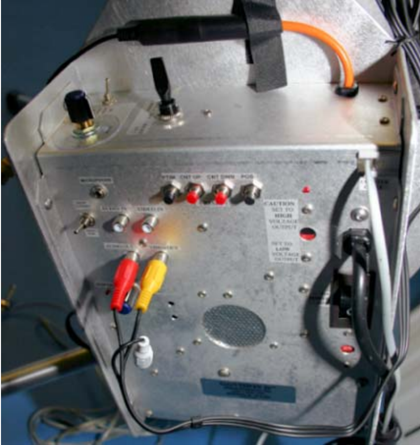
The Deluxe GeoVISION™ system in field use. Note the push pole attached to the front to provide additional stability in deep boreholes.
